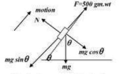
... The body moves with starting velocity 784 cm/sec. and acceleration - 588 cm/sec<sup>2</sup>.
